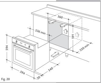
To ensure internal ventilation, aeration channels must be provided as illustrated in the figures 21 and 22.
